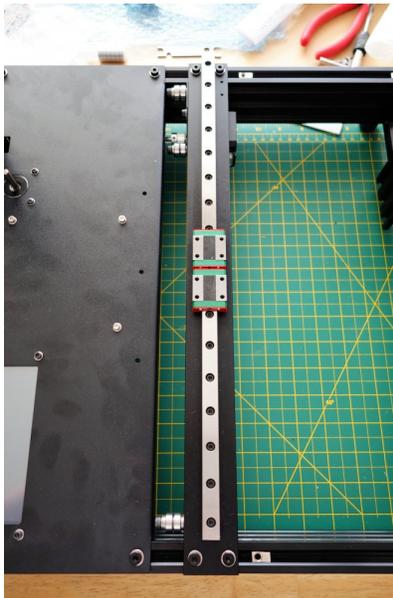
3. Align the assembly so there is about a 1mm gap between the idler screw head and the bend on the Top Deck Left Assembly and tighten.
