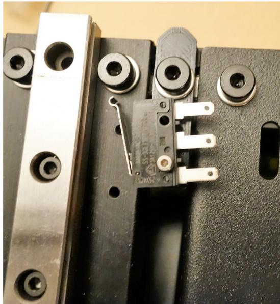
5. The endstop wires are provided with the RAMBo board, they are black and white, with spade connectors on one end, and a keyed connector on the other end. Connect them to the switch outside
