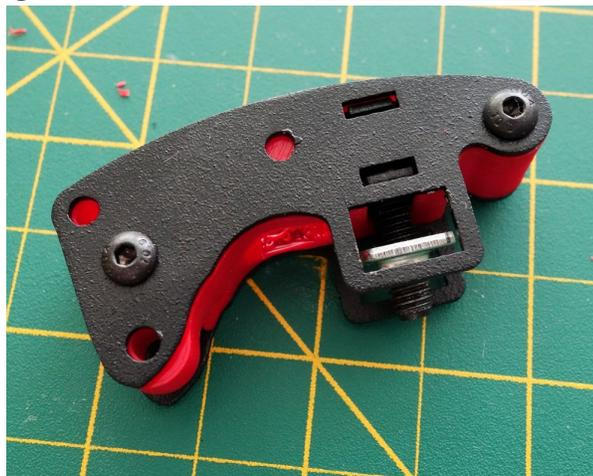
6. Install the small bearing using two M3 Washer to center the bearing to the small filament guide hole in the printed plastic part. Use a **M3×18 SHCS** screw and nut to secure the bearing and washers as shown.
