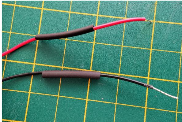
9. Hook the extension wire with the thermistor leads, and slide the ferrule over it. Make sure the ferrule goes a bit over the extension wire insulation. Trim, or bend over the excess leads.
