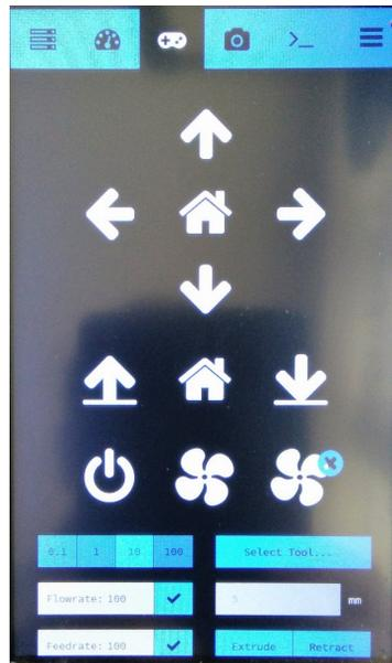
✿ If the control buttons are greyed out, the RPI is not connected to the printer, or there is a fault with the thermistors, see steps 3 and 4.
