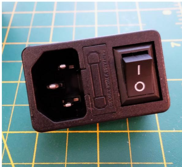
2. Install the fuse into the IEC
