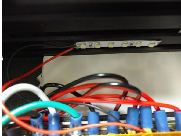
5. Remove the adhesive backing paper off the led strip and stick it to the extrusion as shown in the step above.
