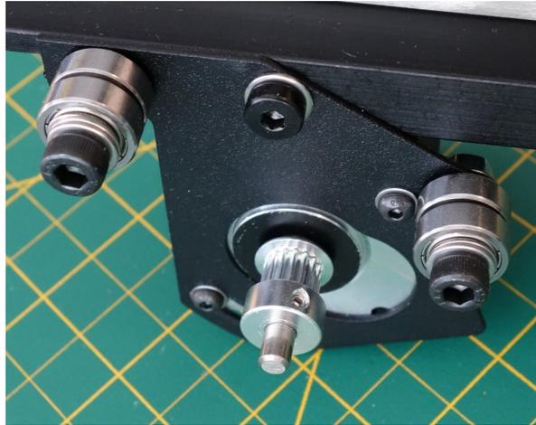
3. All three Idlers will Install in the following order: **M5 × 20 SHCS** > Zero or more **M5 Washer** as needed > **605zz Bearing** > **M5 Washer** > **605zz Bearing** > **M5 Washer** > **Y Motor Mount** or **Machined Y Plate**. The two upper idlers will screw directly into the tapped holes on the Machined Y Plate. The lower idler will screw into an **M5 Nut** Use as many washers below the screw head as needed to keep the bearings snugly in place (probably 2-3).
