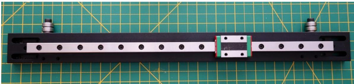
! Handle the assembly carefully after this point. Until it is fully installed, the cars can come off the end of the rail. A couple small strong magnets placed on each end of the rail can keep the blocks from sliding off.
