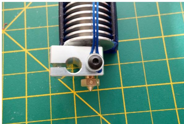
13. Insert the heating cartridge into the heatblock, and secure it with the supplied BH 3×10.
