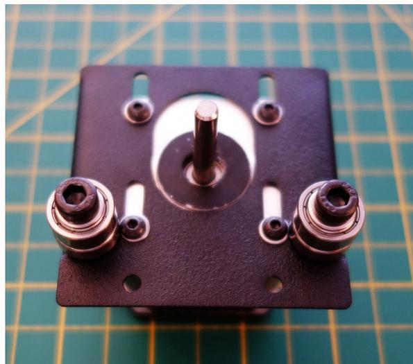
3. Install the pulley, leaving about 1-2mm between the bottom of the pulley and the top of the motor mount plate. Install it with the set screw end of the pulley toward the motor (The opposite of how it pictured). Be sure one of the pulley set screws is aligned with the flat of the motor shaft.
