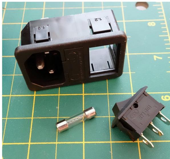
1. Install the switch into the IEC. Note the orientation of the switch, steps 3 and 4 depend on it.
