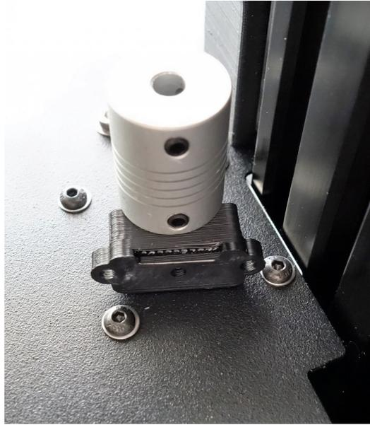
2. Tighten the set screws, making sure one of them is against the flat of the motor shaft.
