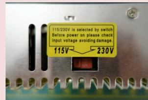
Make sure to set the PSU to the appropriate voltage!
