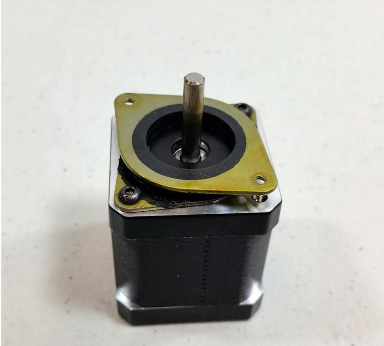
2. Install the **Stepper Motor Assembly** using **2 M3 × 6 BHCS** and **2 M3 Washer**. Two of the slots of the motor mount plate will not be used. Mount it in the position closest to the idlers. Make sure the port on the motor where the cable connects faces the rear of the printer.
