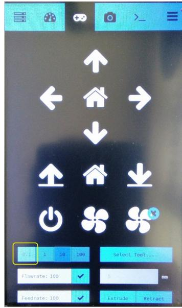
6. Press the **Arrow down** button to lower the Z axis until the nozzle is touching the paper. You can move the paper around while doing this until the paper drags under the nozzle.
