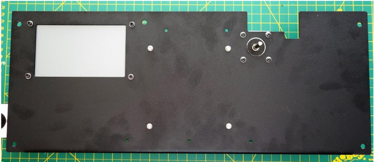
7. The kit comes with a number of printed clips for easier wire management. Those attach to the deck plate with **one M3 × 10 SHCS**, **one M3 Washer** and **one M3 Nut** each. You will install 3 along the “inside” and two along the “outside” edge of the RAMBo.
