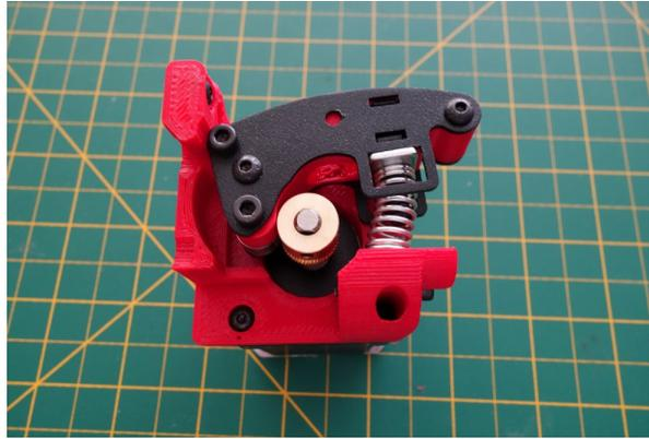
9. Align the brass hob to the filament hole in the arm, and tighten the grub screw against the flat of the shaft.
