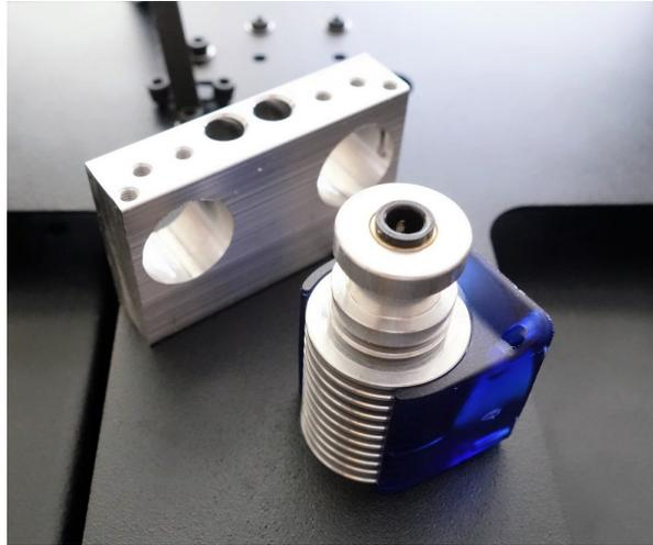
2. Install the Aluminum hot end block to the carriage with **two M3 × 10 SHCS** inserted into the deep holes that are center front of the block.
