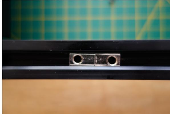
2. Align the M5 Post Install Nut with the holes in the Y Axis Assembly and mount with **4 M5 × 10 SHCS** and **4 M5 Washer**. Leave slightly loose.
