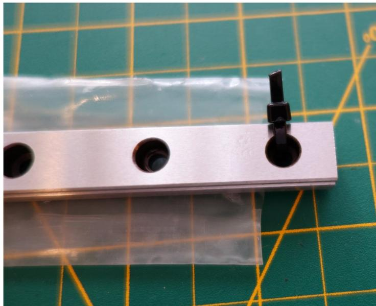
2. **DO NOT REMOVE THE BLOCK.** They are not designed to be removed from the rail.
