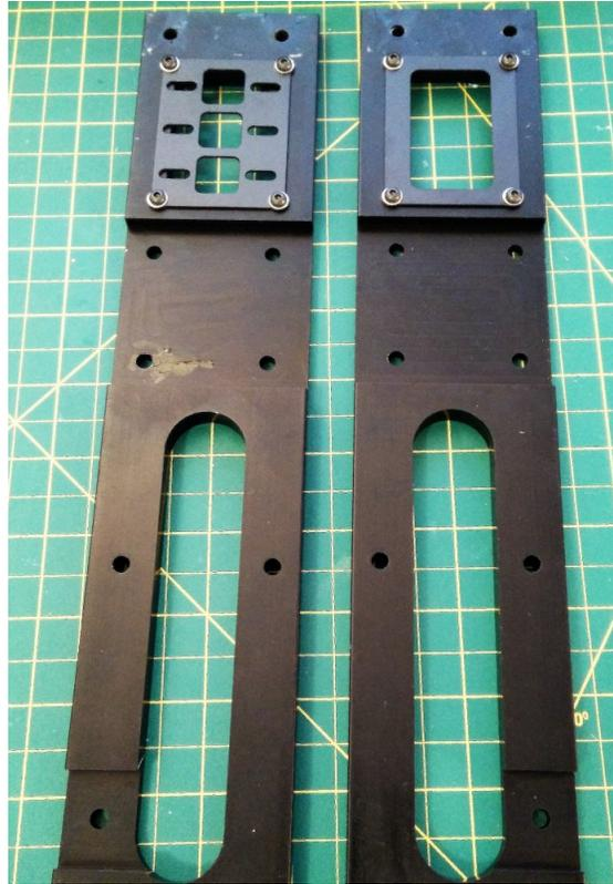
3. Loosely assemble the side plates to the 400mm extrusions using **8 M5 × 16 SHCSs** and **8 M5 Washers**. **Do not tighten the screws yet.**
