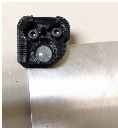
3. Install the **Y Belt Offset** using **two M3 × 10 SHCS** with **M3 Washers**. Note the screws now go up from the bottom into the tapped holes on the Y Carriage Plate.
