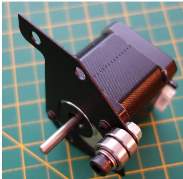
4. Locate the two 5mm tapped holes on the side of the Machined Y Plate and attach the Y motor plate using an Idler Bearing assembly and an **M5 × 10 SHCS** with a **M5 Washer**. See the images below for clarification.
