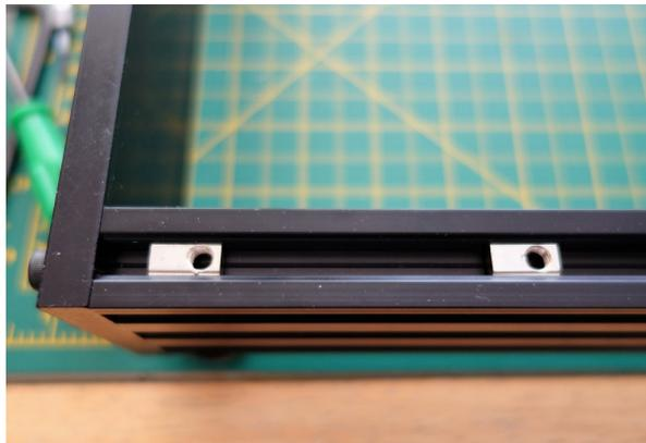
2. Align the M5 Post Install Nut with the holes in the Top Deck Left Assembly and mount with **4 M5 × 8 SHCS** and **4 M5 Washer**. Leave slightly loose.
